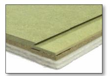
Trim Defender 21 is designed to be laid directly on top of an existing timber floor construction in a broken bond pattern with all joints glued and perimeters sealed using 23mm x 5mm Perimeter isolation tape.
