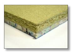
Trim Defender 28 can be laid directly onto a concrete floor or on top of an existing timber floor constructionin in a broken bond pattern with all joints glued and perimeters sealed using 30mm x 10mm Perimeter isolation tape.
