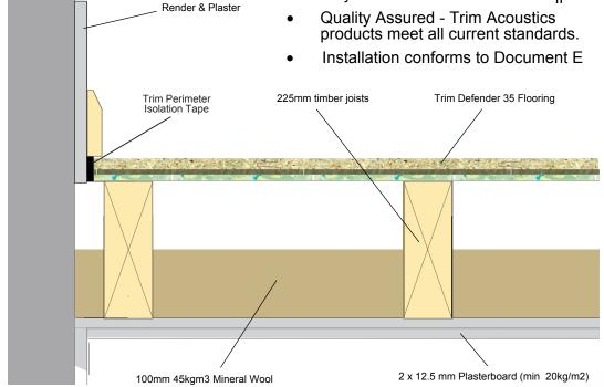
Trim Defender 35 is the perfect choice where the existing floor is in poor condition and needs to be replaced. Defender 35 gives you your structural floor and acoustic floor all in one, so saving time and money compared to laying two separate floors.
