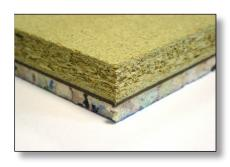
Trim Defender 35 should be laid directly onto the joists in a broken bond pattern with all joints glued and perimeters sealed using 37mm x 10mm Perimeter isolation tape.
